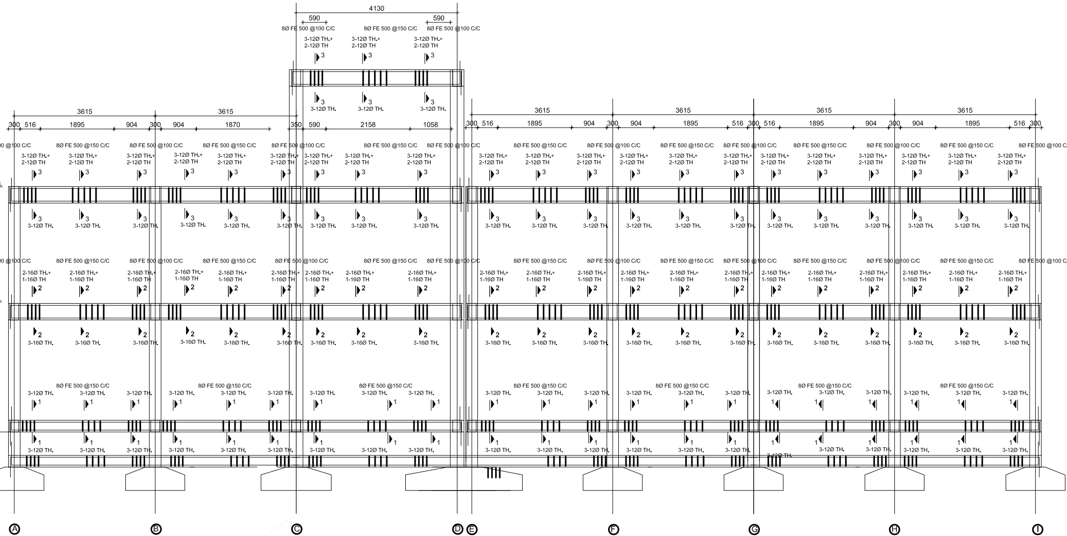
REINFORCEMENT DETAILING FOR GRID 1-1, 2-2 AND 3-3 SCALE 1:50
